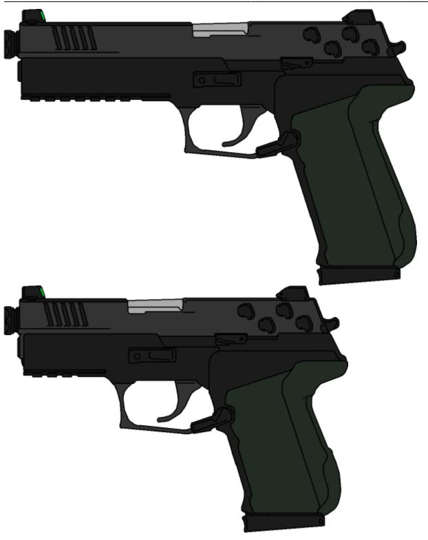
Constructed using all steel. Slide is set into the actual frame of the pistol. Serrations at the front and rear of the slide. Accessory rail under the frame towards the front. Trigger guard is wide and spurred at the bottom, pointing forward. Magazine release built into the trigger guard toward the rear. Slide catch lever on the frame, above to the left of trigger. Slide stop lever on the frame near the top, to the right of the trigger. Decocker is a button on the rear of the slide.
