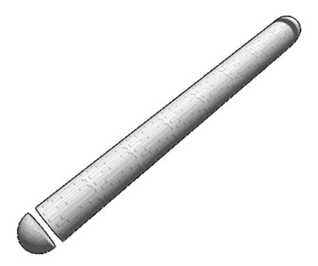
Located at both of the ends of each tank is the tank support dome. These consist of a series of pumps, filters and thermal control systems. These include the ports that is used to fill the inner tank. The filter system is used to purify impurities from water. The thermal system is intended to keep the contents from freezing which could damage the tanks.
