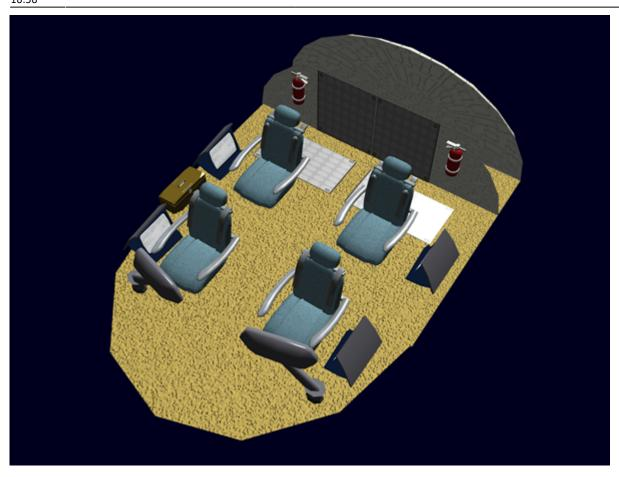
There are two in-floor storage areas in the rear of the shuttle where two *EM-G19* - *Survival Kits* are typically stowed.
