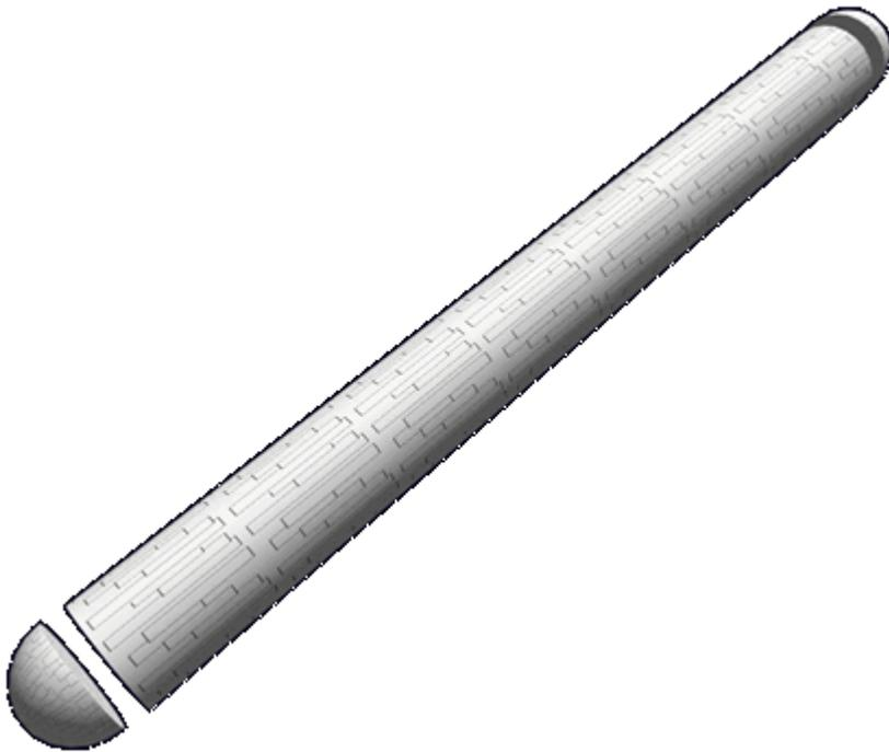
Located at both of the ends of each tank is the tank support dome. These consist of a series of pumps, filters and thermal control systems. These include the ports that is used to fill the inner tank. The filter system is used to purify impurities from water. The thermal system is intended to keep the contents from freezing which could damage the tanks.
