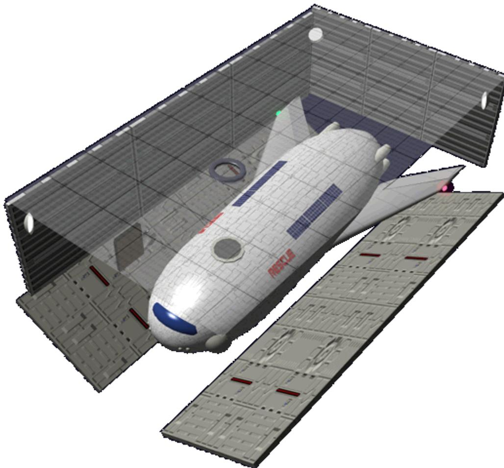
A secured maintenance door is present on one of the interior walls to allow technicians to enter the bay and service the craft. There are four interior lamps used for maintenance and during launch.
