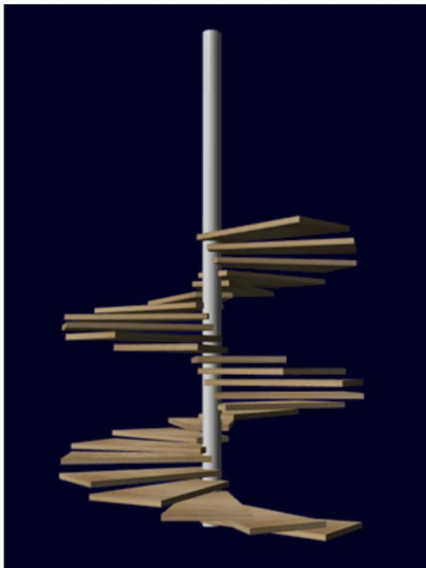
The staircase has steps that are two meters wide which allows people to go up and down at the same time. Clearance is 2 meters as well. The stairs surface depends on the customer's preference.
