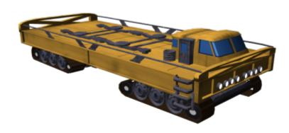
The Balaena is a simple design, long and wide with a small cab at the front centre, containing two work stations and seats for the crew. The majority of the vehicle is dedicated to acting as a platform to attach various equipment and is flat with several power connection ports and hydraulic control cables which are connected to the chosen equipment allowing it to be controlled from the cab.
