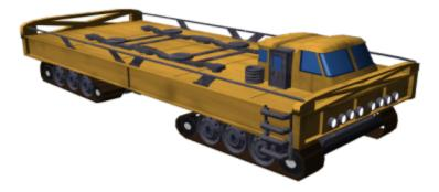
The Balaena is a simple design, long and wide with a small cab at the front centre, containing two work stations and seats for the crew. The majority of the vehicle is dedicated to acting as a platform to attach various equipment and is flat with several power connection ports and hydraulic control cables which are connected to the chosen equipment allowing it to be controlled from the cab.
