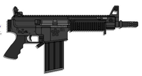
The rail that runs the length of the carbine's top is rather boxy and houses the gas piston system, opting for twin folding charging handles on both the left and right, situated above the handguard. While a stock is not included with the rifle by default it does feature hardware designed to accept M3 compatible stocks should the owner desire to install one.
