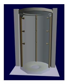
The showers have nine shower heads, water intensity can be varied from normal spray to massaging pulses. The showers are voice command controlled, for temperature, pressure, number of shower heads and nozzle setting. When the water is turned off two blowers engage and force warm air at the occupant, this helps to drive the airborne moisture out as well as removing the majority of water from the occupants body.
