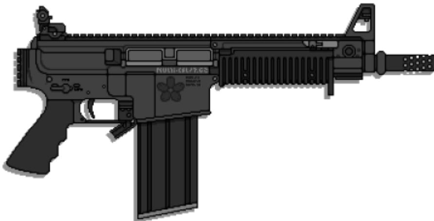
The rail that runs the length of the carbine's top is rather boxy and houses the gas piston system, opting for twin folding charging handles on both the left and right, situated above the handguard. While a stock is not included with the rifle by default it does feature hardware designed to accept [M3 compatible](#) stocks should the owner desire to install one.
